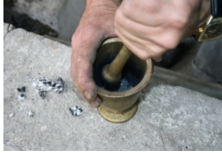
Image 30: Pulverizing the Niello
