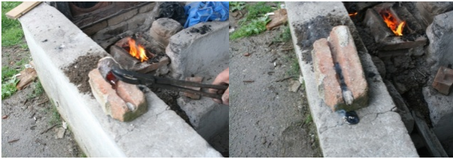
Image 26: Pouring the melted Niello to the iron mold
