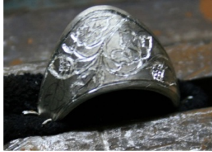
Image 28: Patterning and Carving the silver surface
