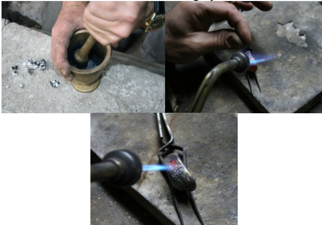
Image 29: Pulverizing then Spreading the Niello and after heating the silver
